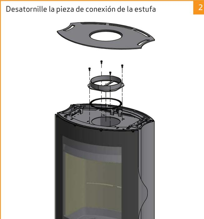
The diagram shows the stove connection piece being removed. The piece is shown being unscrewed from the top of the stove, with the screws and the piece itself being lifted away.
