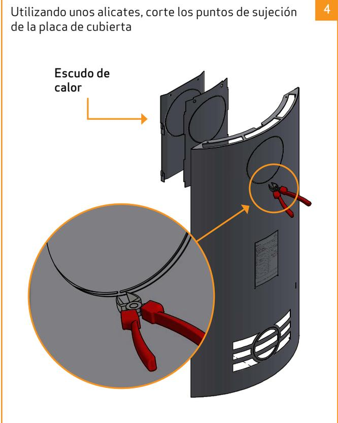
The diagram shows the use of pliers to cut the attachment points of the back cover plate. A circular inset provides a close-up view of the pliers cutting through the metal at the attachment points. The thermal shield is also labeled.
