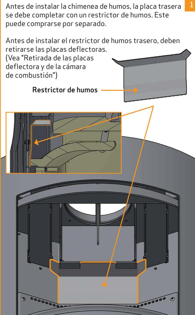
The diagram illustrates the installation of a smoke restrictor. It shows a top-down view of the stove's rear panel with a rectangular restrictor being placed into a designated slot. An inset diagram shows the removal of deflector plates from the combustion chamber area.
