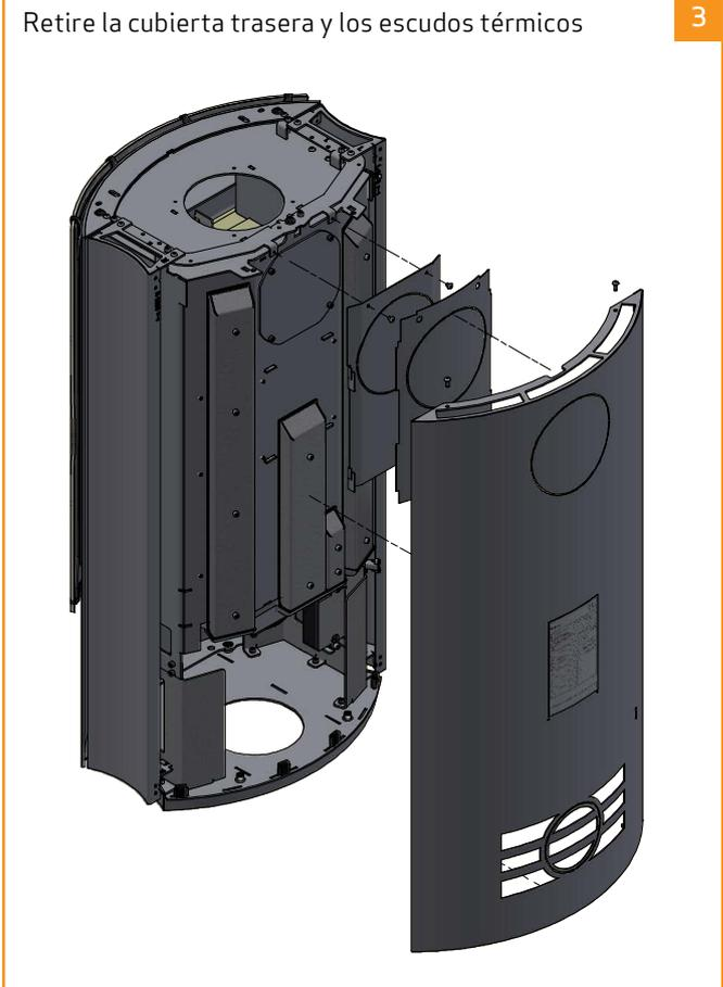
The diagram shows the back cover and thermal shields being removed from the stove. The back cover is shown detached and leaning against the stove, revealing the internal components and the thermal shields.
